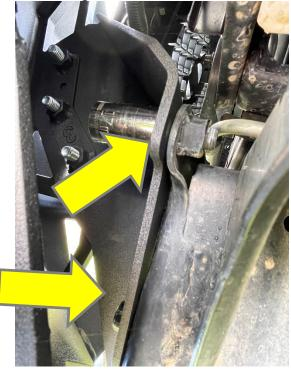
5. Attach lower frame mounts to frame mounts with the head of the bolt to the inside of the truck using bolts from hardware kit 60K-56-0001. Leave all hardware hand tight. Make sure to use washers and lock washers. Use hardware kit 60K-56-0209 to fasten lower frame mount to the truck.
