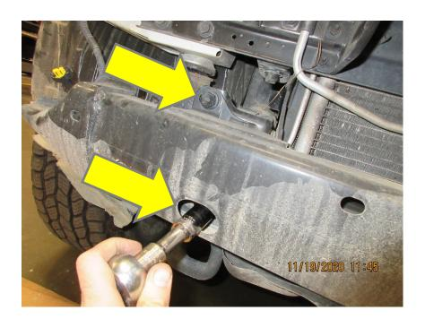
10. Remove 2 bolts with a 17mm socket from tow hook and remove tow hook. Set bolts aside to be reused.
