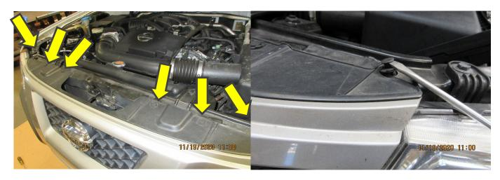
2. Using access gap between radiator and grille, remove 5 plastic retainers attaching bottom of grille to top of bumper. (2 additional plastic retainers not pictured)
