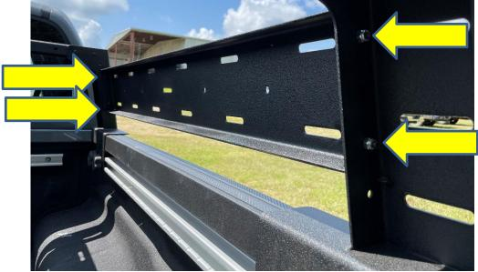
6. Using an 11mm socket or wrench and a T30 bit, tightly fasten all hardware. An impact driver will make this a quick and easy task. Use wire loom clips in install kit 60H-56-0278 to securely hide any wiring.
