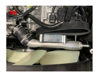
Re-connect the temp sender loom.
