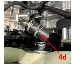
**4.e)** Insert the radiator hose assembly into position and then insert into the reducer hose.
