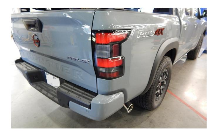
Note: When you first start your vehicle after the installation of your new NISMO Performance Exhaust System, there may be some smoke and fumes coming from the system. This is a protective water based coating used in the manufacturing of mandrel bent performance exhaust tubing. This is not a problem and will disappear within a very short period of time after the exhaust has reached operating temperatures.
