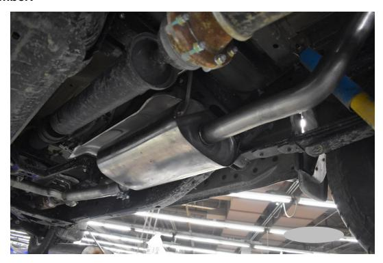
STEP 4: Remove the rubber mount for the tailpipe from the frame. Slide a 2.5" clamp over the muffler outlet pipe. Work the tailpipe over the rear axle and slide the expanded inlet over the muffler pipe. Slide the rubber mount over the tailpipe hanger and reinstall to frame.
