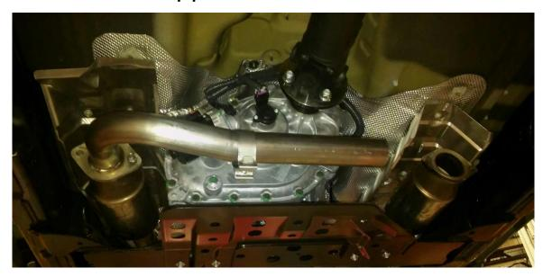
STEP 2: Align the Passenger side y-pipe with the drivers side pipe and passenger side catalytic converter, re-using the OE gasket, and tightening the nuts a few turns to keep the piping loose for fit-up. Slide the hanger through the rubber mount on the cross member. Note: removing the isolator mount from the frame and reinstalling may help make the job be easier.
