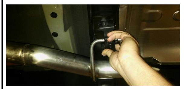
Note any orientation marks on the bracket if removed and reinstalled.
