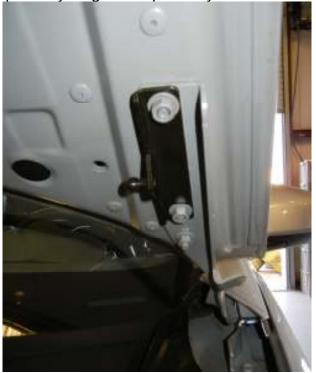
4. Now that you have all the brackets installed you can move onto the struts. The struts use 2 different style ends for installation, a removable end with the additional pin lock (for the hood side) and a positive lock end for the front side. \*Do not install the sloped end of the piston rod onto the hood bracket. It cannot be removed from the ball once installed! Snap this positive lock end onto the lower ball stud at the front of the brake or battery covers.
