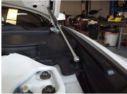
**5.** Now, make sure you do not have the lock pins installed, align the ball end over the ball stud and snap into place. Install the lock pin and you are finished.
