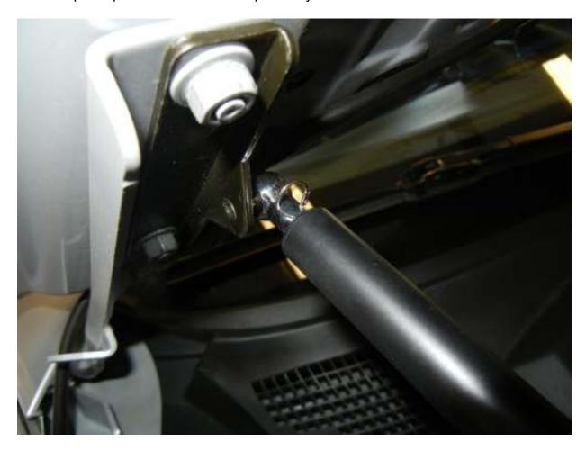
To get the lock pins installed pass the straight part of the pin through the ball end and rotate it around until it snaps into place. Now you are all finished.
