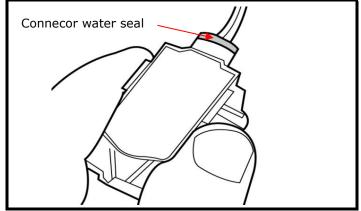
2.6) Reinstall connector water seal into the back of the LOGO lamp body
