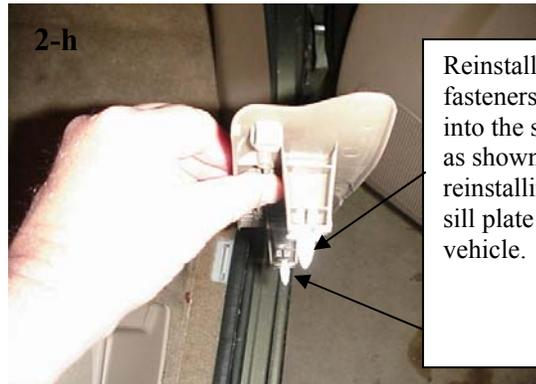
Reinstall the fasteners back into the sill plate as shown before reinstalling the sill plate on the vehicle.
