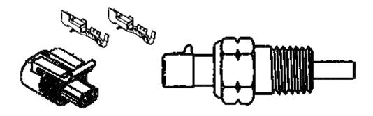
**Housing Material:** Brass with 3/8" NPT Thread (Torque to 25 Ft-Lbs) **Elec. Termination:** Integral weatherproof connector, Includes mating connector with 2 terminals.
