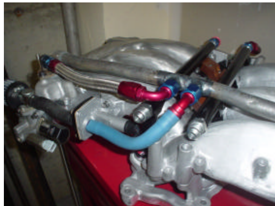
Figure 3 — Idle air plumbed with AN hose fittings
