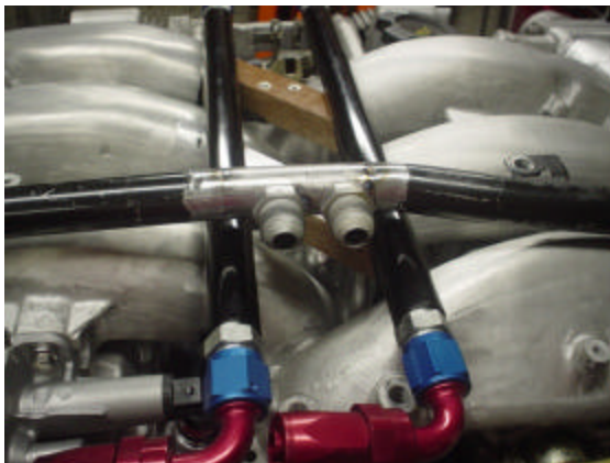
Figure 2 — Modified balance/crossover tube
