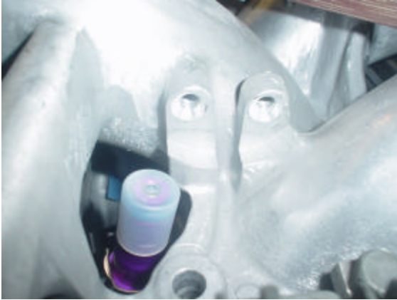
Figure 4 — countersunk bolt holes
