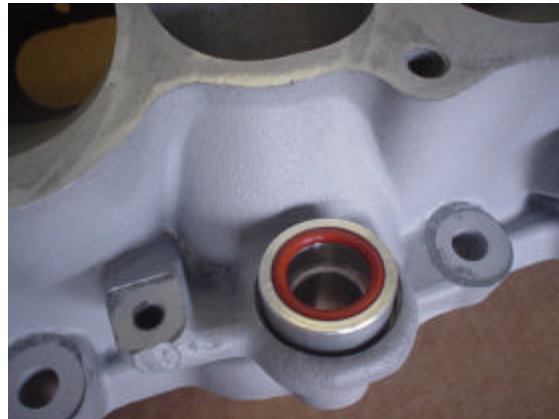
Figure 7 — std. depth injector adapter and cushion
