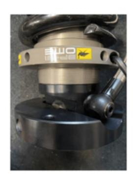
4. Loosen the pinch bolt using a 5mm Allen key.
