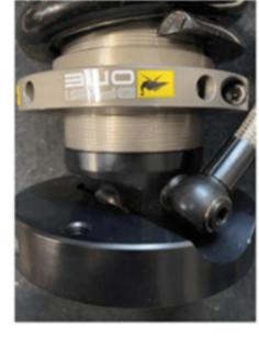
3. Compress the coil spring until the threaded spring preload ring is not in contact with the coil.
