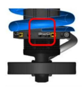
Position the end of the coil such that it is opposite the hose fitting.
