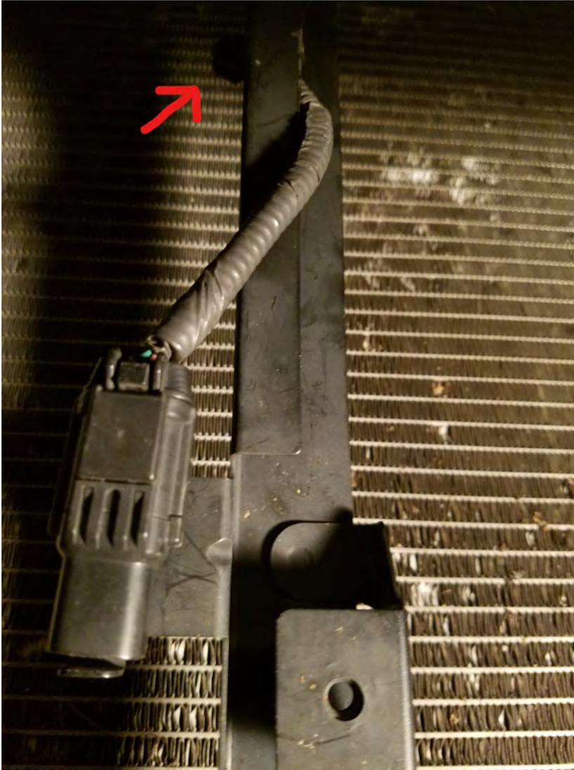
(The harness should be clipped back into the same hole on the opposite side just like seen in this photo to the left)
