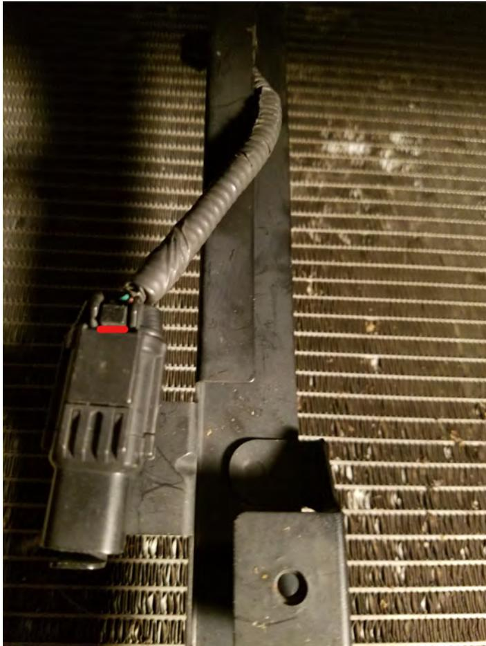
**STEP 5: Switch ambient temperature clip from the passenger side to the driver side as pictured below**
