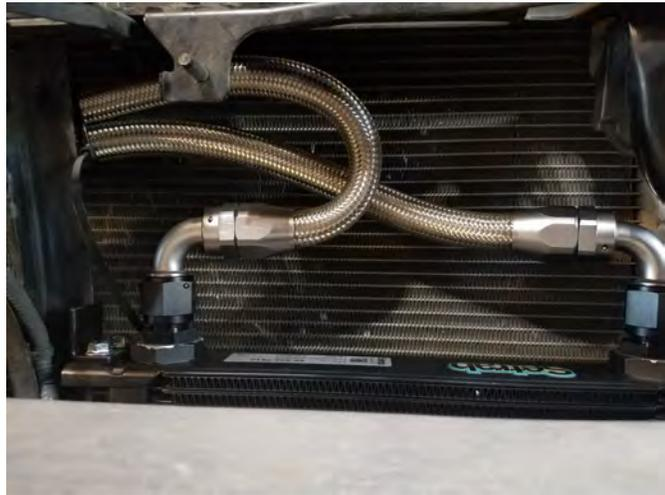
After setting up the oil cooler for installation, set it back down below the vehicle while we move on to installing the Air-Guide.
