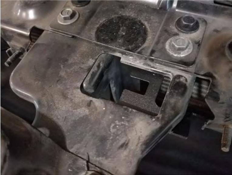
Make sure that both upper sides of the air guide are even and snug the body nuts on the underside of the brackets once the hood latch relief is aligned as such. Check clearance by slowly setting the hood down and watching it as it clears. Adjust accordingly and then with a 10mm socket on a 1/4 drive extension, ratchet the two body nuts on the bottom side of the core support. We are done here for now.
