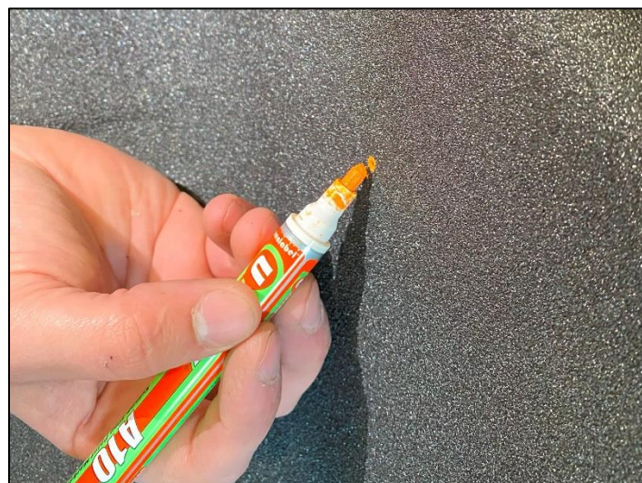
Using a paint marker to mark the center punch
