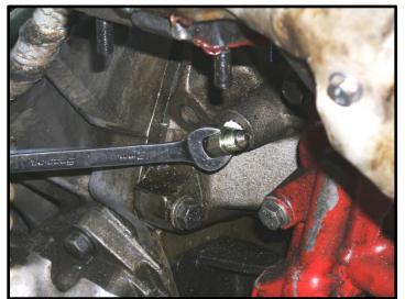
9. Attach the straight end of passenger side oil feed line to 90° fitting. Attach the other side with brass restrictor fitting, to feed port on turbo, routing the line under the turbo (as shown).
