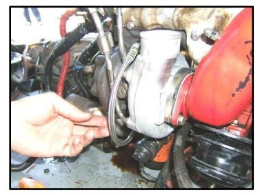
10. Using the banjo bolt from the passenger side feed line (**NOT** the "K-Bolt" pictured below from the OEM driver feed line), attach the driver side line to the engine block (as shown).
