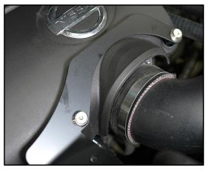
15. With a clamp on each end, attach hoses coming out of the tee's to the catch can (as shown below).
