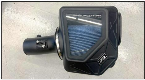
20. Position intake tube and airbox assembly into vehicle, making sure the grommets on the bottom of the air box line up with the studs on the chassis (studs shown with arrow below). Then press down on the airbox to seat the grommets onto the studs.
