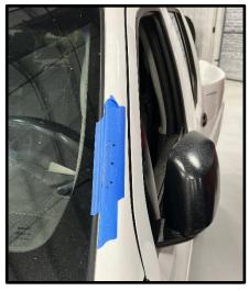
23. Pilot drill the hole, then drill out to fit supplied rivets.
