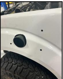
17. We found that the self-adhesive foam isn't necessary and will require some trimming for a perfect fit. Without trimming, the main snorkel body would not sit flush. We opted to install without it. If you would like a perfect fit with the foam, the following pictures show where we had to trim.
