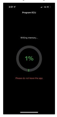
6. When prompted, turn the ignition off. Wait a few seconds, and when prompted again, turn the ignition back on. **DO NOT** start the engine during this time, just turn the key to the "ON" position. For push button cars, ensure the brake pedal is not depressed when doing this.
