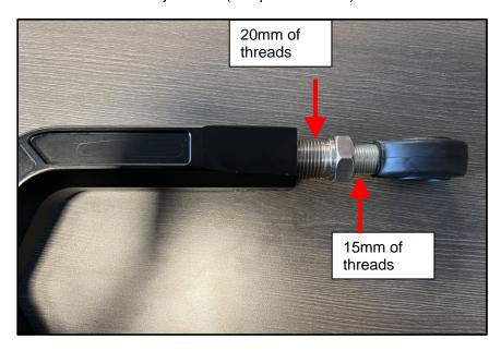
18. Once the Z1 arms are the same length as the OEM arms, tighten the (2) Allen head pinch bolts, switching back and forth until both bolts achieve **20ft-lbs**. Then, tighten the jam nuts on the heim-joints against the double adjusters with an adjustable wrench or 28mm.
