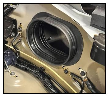
11. Remove/pull back front of driver fender liner. Install fender grommet velocity stack onto lip of fender grommet inside wheel arch (as shown). Reinstall fender liner.
