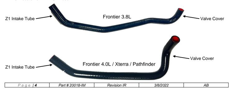
17. Using the OEM hose clamp, attach Z1 PCV hose end with longer bend to valve cover (as shown).
