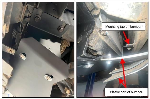
7. Loosely secure the front mounting tabs on the skid plate to the mounting tabs on the front bumper with (2) M6 x 16mm bolts and washers. On Xterra (shown below) there will be access holes in the front bumper allowing you to install these bolts. On Frontiers you will need pry the bottom of the bumper away and use a wrench to access these.
