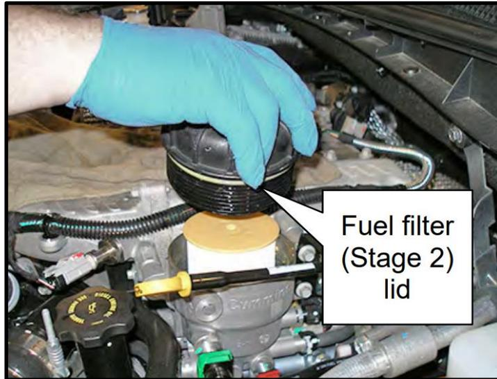
10. The fuel filter element will come out with the lid. Remove the old filter.
