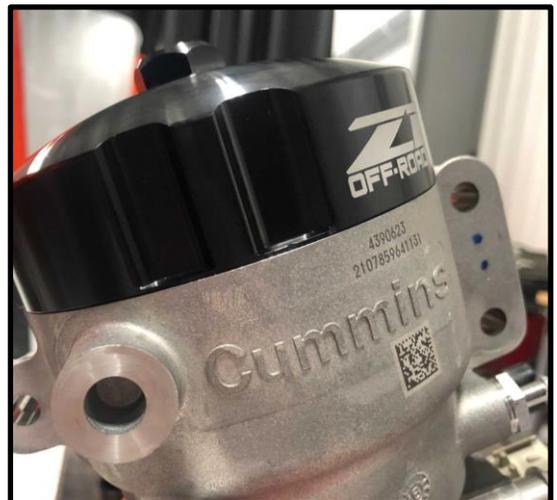
17. Start vehicle. While at idle, check for leaks or faulty operation of fuel filter cap.
