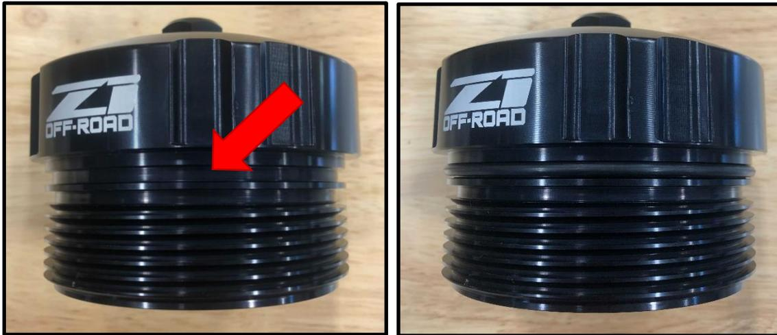
13. Locate and install the fuel filter element onto the standpipe in the fuel filter housing.
