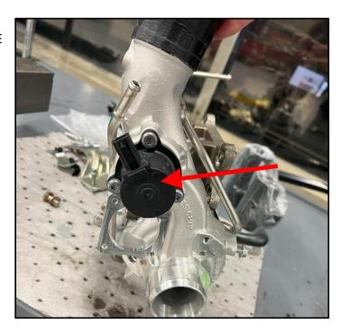
16. Re-using your OEM clamps, install Z1 BOV couplers. Refer to figures 1 and 2 for proper orientation. Depending on if you have stock or Z1 upgrade turbos you will receive different BOV silicone couplers, each coupler should have a small label indicating its part number. Stock turbo customer will receive 22057-B (passenger) and 22057-C (driver). Z1 VRX70 customers will receive 22057-D (passenger) and 22057-C (driver).
