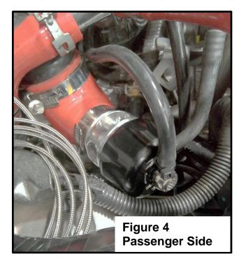
HKS customers: Install the HKS BOV's into the silicone couplers (as shown below).
