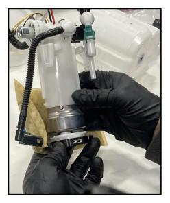
28. Then install the smaller piece into the slots on the pump assembly housing, making sure both ends of the clamp piece are in a slot (as shown below). Begin to thread the (2) M5 screws through both pieces to secure them together. Add a dab of red Loctite before final tightening.
