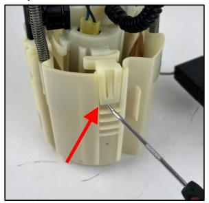
19. Release the (3) locking tabs securing the fuel pump strainer to the bottom of the fuel pump and then remove the strainer and set aside.
