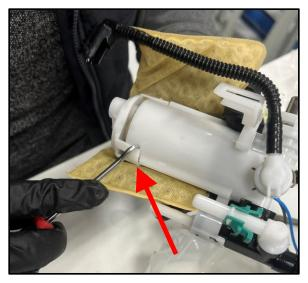
20. Remove the OE fuel pump from the pump assembly housing. Once removed disconnect the electrical connector at the top of the OE fuel pump.
