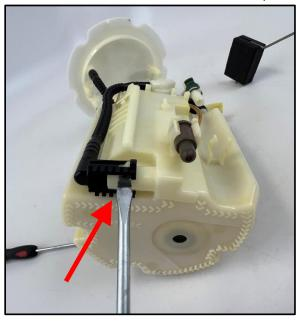
18. Release the (3) tabs securing the pump assembly housing to the lower basket (1 tab shown below). Then lift up to remove the pump assembly from the basket.
