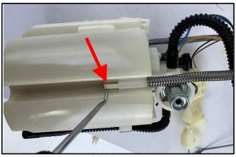
15. Once the top and bottom halves are separated, disconnect the (3) electrical connectors on the bottom side of the top hat. Take note or a picture of the two gray connectors as they can be incorrectly installed later.
