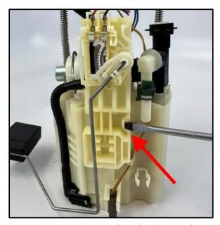
17. Release the locking tab on the hose at the bottom of the fuel basket (as shown below).
