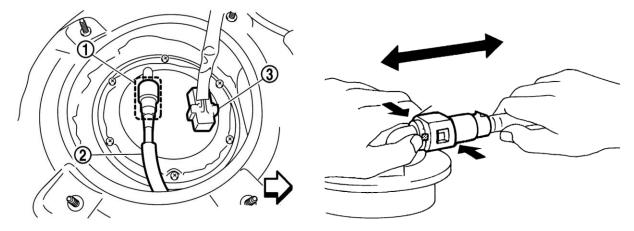
9. Using an 8mm socket, remove the (6) M5 screws securing the OE fuel top hat collar to the fuel tank.
