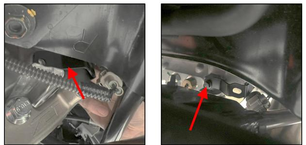
11. Performance Model 2023+ Z Owners: Secure the wiring harness to the new bracket (as shown below).
