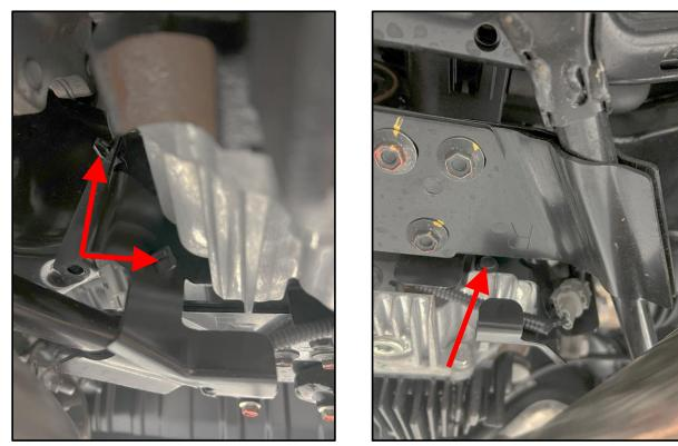
4. Remove (2) bolts on the bottom right of the rear differential housing cover (as shown).
