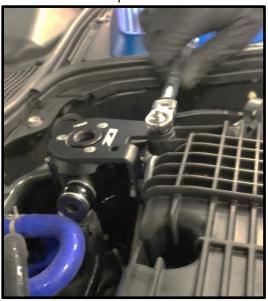
Note: If your plenum does not have a stud in this location, please use the supplied M6-1.0 x 10mm flanged bolt to secure the bracket in place.
