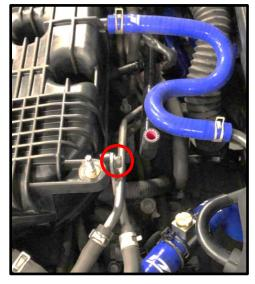
12. Locate catch can backet. Place catch can bracket onto stud next to bolt removed in step #12. Thread bolt from previous step back into the same mounting hole securing the catch can bracket in place. If your plenum does not have a stud in this location, please use the supplied M6-1.0 x 10mm flanged bolt to secure the bracket in place.
