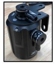
15. Thread the supplied M6 lock nut onto stud on top of catch can bracket.
