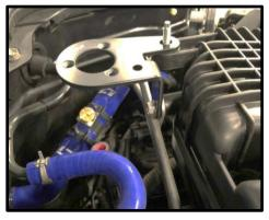
13. Locate Z1 Catch Can, (3) M4 screws, and (1) 2.5mm Ball-End Hex Screwdriver. Attach bracket to top of catch can using (3) M4 screws and the supplied 2.5mm Ball-End Hex Screwdriver in the same orientation as pictured below. Be sure the outer screw under the access hole in the top of the bracket is accessible.
