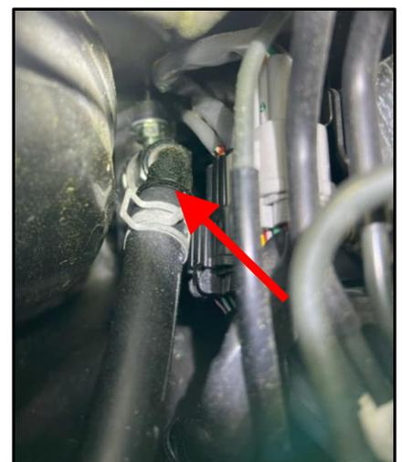
18. Install the assembled Z1 Tilton Clutch Master Cylinder into the vehicle with the (2) studs on the bracket going through the OEM holes in the firewall that the OE cylinder was removed from in step # 13.
