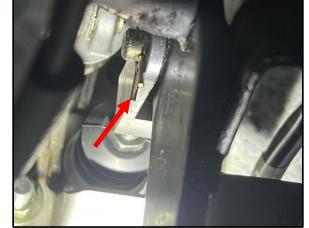
12. Using a 12mm socket/wrench, remove the (2) nuts securing the OE clutch master cylinder to the firewall (shown below). You may need to use a combination of some extensions and a universal swivel socket for easier access.
