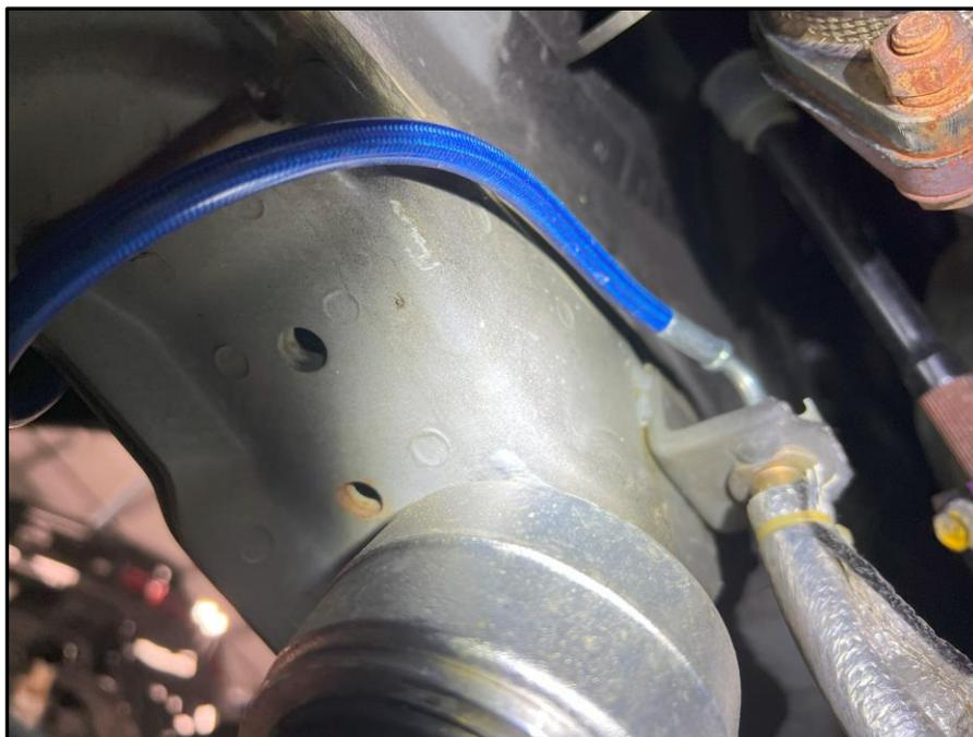
35. Reconnect the OE clutch reservoir hose to the push-on fitting on the Tilton clutch master cylinder, secure with hose clamp.
