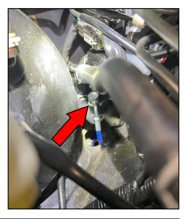
31. If applicable, install the new Z1 clutch line into the OE clips in the wheel-well. Then using the OE screw that was removed in step # 25 secure the bracket on the Z1 line to the wheel well (shown below).
