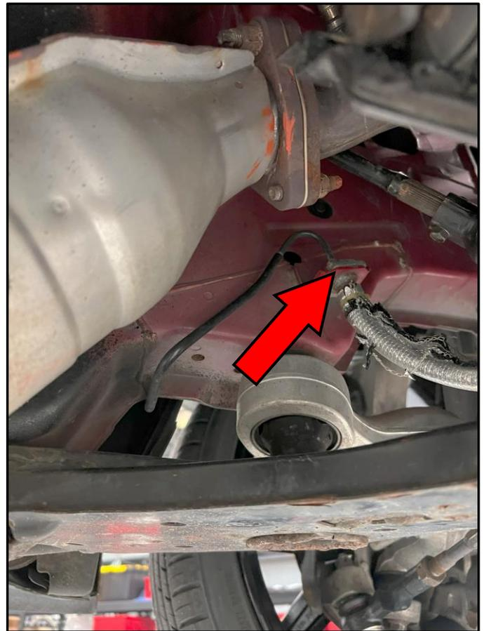
26. Remove the upper half of the hardline by twisting/wiggling the line to pull it out of the brake compartment. The rubber grommet on the wheel-well will likely get removed with the hardline, if so remove the rubber grommet to transfer over to the new Z1 clutch line.
