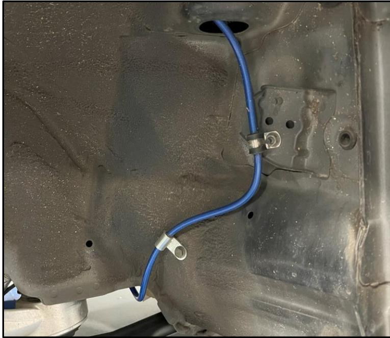
32. Using the supplied cushioned P-clamp and OE nut that was removed in step # 25, secure the line to the stud in the wheel well that held the OE damper (shown above).
