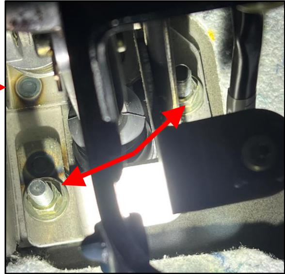
13. Go back to the brake compartment and fully remove the OE clutch master cylinder and reservoir assembly.
