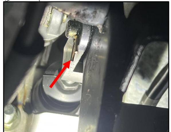
12. Using a 12mm socket/wrench, remove the (2) nuts securing the OE clutch master cylinder to the firewall (shown below). You may need to use a combination of some extensions and a universal swivel socket for easier access.
