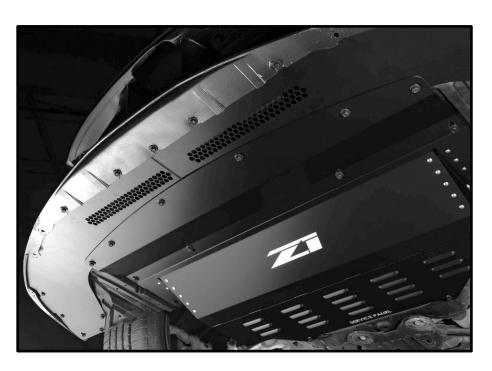
6. Attach the front of the extension panel to the bottom of the front bumper cover using (5) supplied M6 SEMS screws (as shown above).
