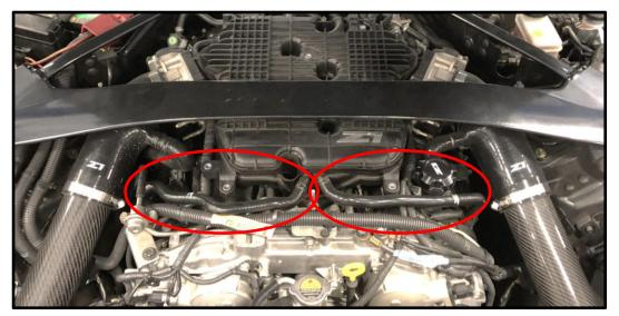
9. Using the 40mm bolt, attach driver side catch can assembly to radiator core support where bolt was removed in step #7.
