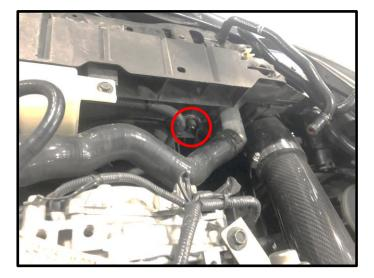
8. Remove both OEM PCV hoses, running from each valve cover to the front of the intake plenum (circled below).
