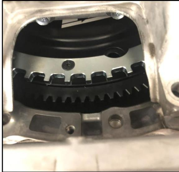
13. Using the access hole, with a dab of Loctite on each, install the (4) supplied bolts securing the Z1 flex plate to the torque converter. Torque bolts to 38ft-lbs in an X pattern and in steps.
