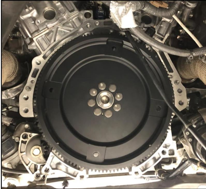
9. With either a ring gear stopper installed or large ratchet on the front of the crankshaft, install the (8) flex plate bolts that were removed in step # 5-6 , diagonally and in steps to secure the flex plate to the engine. Torque bolts to 65ft-lbs. It is highly recommended to add a dab of Loctite to each bolt.
