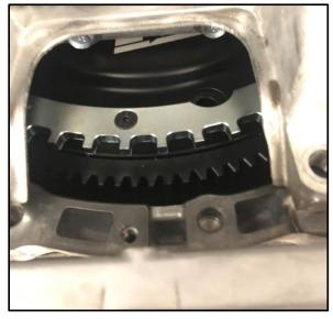
13. Using the access hole, with a dab of Loctite on each, install the (4) supplied bolts securing the Z1 flex plate to the torque converter. Torque bolts to <u>38ft-lbs</u> in an X pattern and in steps.
