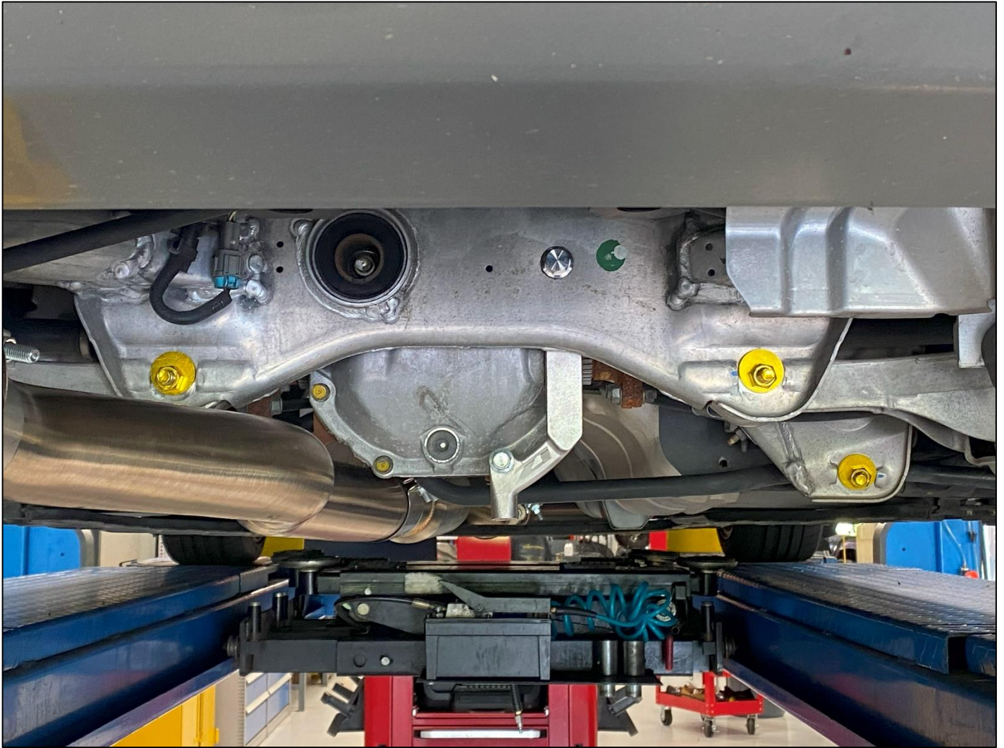
Installed Z1 Eccentric Bolts
