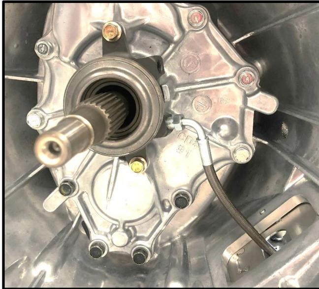
8. Run the clutch line (longer of the two) through the dust shield and thread into the bottom port on the CSC (as shown).
