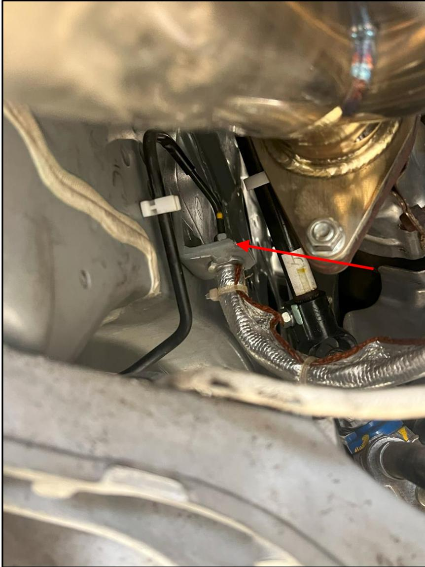
12. Bleed the lines using the bleeder port on the outside of the bellhousing. The “seat” for the bleeder is intended to hold the line in place and only require (1) wrench to open and close the bleeder valve.
