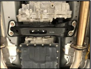
Remove the (4) bolts securing the transmission mount to the transmission. Remove the old transmission mount.
