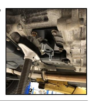
6. Remove the (4) bolts and (2) nuts securing the transmission cross member to vehicle. Remove the cross member and set aside.
