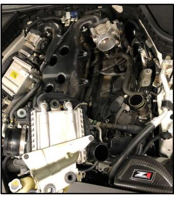
7. Disconnect factory PCV hose. It is attached at the front of the driver side valve cover (next to oil fill cap) and connects to the rear of the intake manifold (next to the driver side throttle body).
