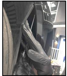
14. Disconnect any electrical connectors attached to the crash bar.
