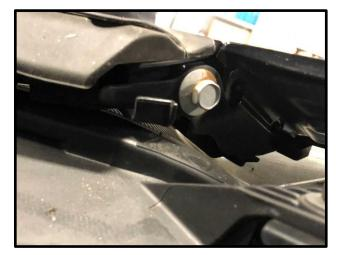
7. Remove plastic clips and peel back front wheel liner to reveal (1) mounting screw at each side of vehicle which mounts bumper fascia to the vehicle (as shown). Remove mounting screws.
