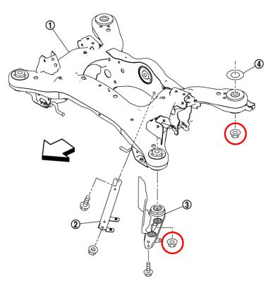
5. It is now time to remove the factory rear differential bushing. To start, we recommend using a body or recpricating saw to cut the middle of the factory bushing out (as shown). Depending on the condition of your factory bushing, you may want to drill into the bushing first to try and remove as much hydraulic fluid as possible (as shown).
