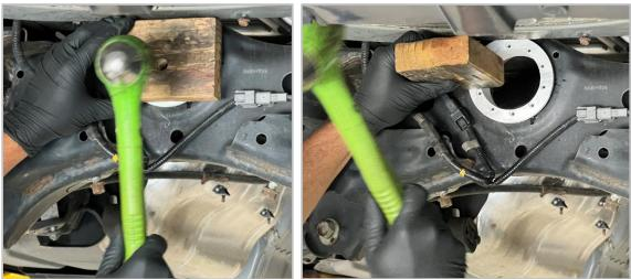
a. Hammer the bushing in evenly. Turn the wood on its side to focus the force on one side if it's going in unevenly.
