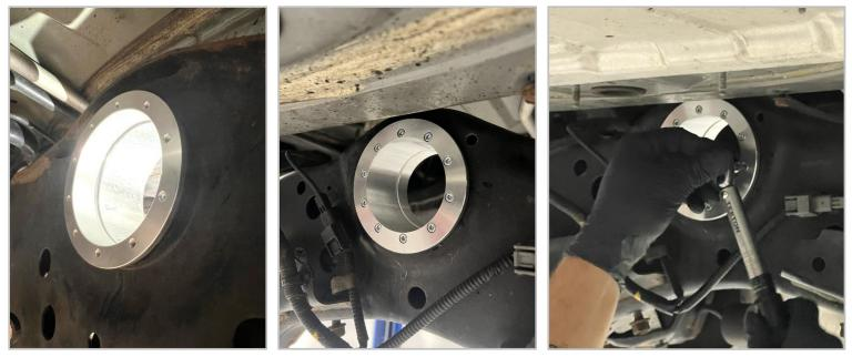
15. Locate the large rear urethane bushing. Install bushing into rear busing sleeve using a rubber mallet. The bushing is slightly tapered on one end to ease with installation, the tapered end should be facing forward.
