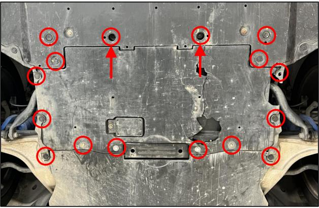
4. Install a supplied SEMS screw into the center 2 riv-nuts on the bottom of the radiator core support (as shown below). The riv-nut locations are shown in the image above with an arrow pointing to their them.
