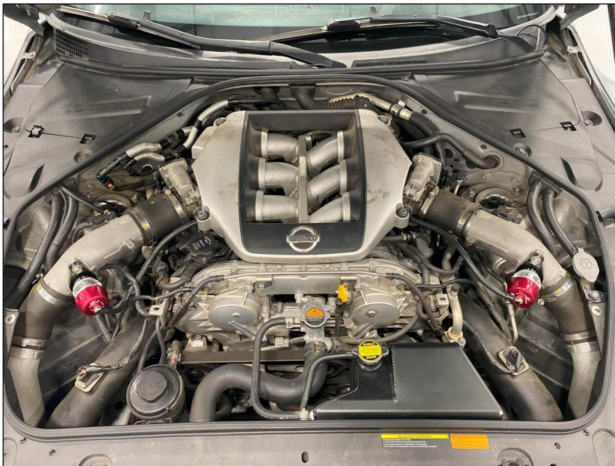
*Installed Z1 GTR Blowoff Valve Adaptors*
