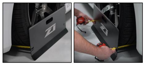
4. Measurements should be taken by comparing the lengths of the (2) tape measures. If the front tape measure is longer than the rear, the vehicle is toed out. If the rear tape measure is longer than the front, the vehicle is toed in.
