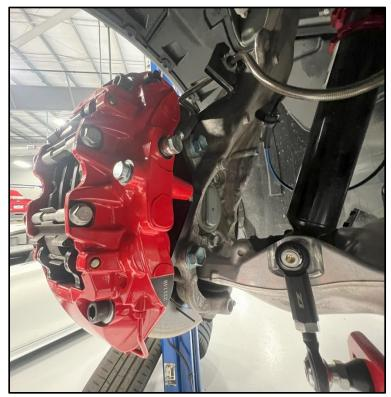
17. Secure the brake line to the rear of the caliper.
