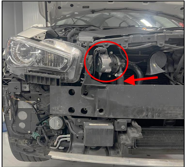
16. Non-Red Sport Models: The outlet hose coming off the first water pump has multiple hose sections with joiners (shown below). Remove the second hose coming off the joiner that goes towards the front of the radiator and connects to another joiner that contains a sensor. Remove the clamps at both joiners and remove the hose. Retain the hose clamps as they will be reused.
