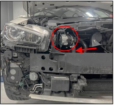
16. <u>Non-Red Sport Models</u>: The outlet hose coming off the first water pump has multiple hose sections with joiners (shown below). Remove the second hose coming off the joiner that goes towards the front of the radiator and connects to another joiner that contains a sensor. Remove the clamps at both joiners and remove the hose. Retain the hose clamps as they will be reused.
