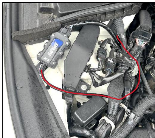
**Note:** The image at left is shown with the grommet and wiring harness already installed. Instructions for those steps are below. The image is to be used as reference for how to route the power cable.
