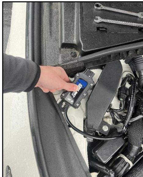
29. While still holding the controller and bracket in the same position, use a phillips head screwdriver to tighten the (3) screws securing the bracket to the controller enclosure.
