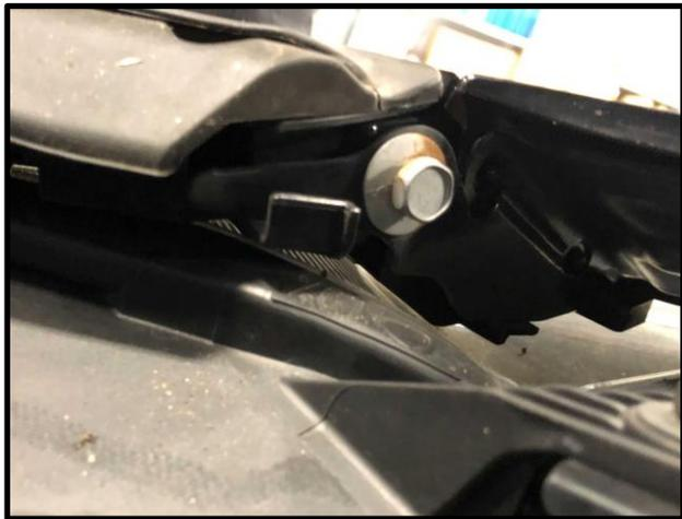
7. Remove plastic clips and peel back front wheel liner to reveal (1) mounting screw at each side of vehicle which mounts bumper fascia to the vehicle (as shown). Remove mounting screws.
