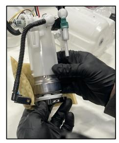
29. Then install the smaller piece into the slots on the pump assembly housing, making sure both ends of the clamp piece are in a slot (as shown below). Begin to thread the (2) M5 screws through both pieces to secure them together. Add a dab of red Loctite before final tightening.
