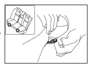
3. Pull up on the sound deadening cover and move to the side. Then remove the clip that holds the fuel pump wiring harness to the stud (shown with arrow below).
