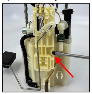
18. Release the locking tab on the hose at the bottom of the fuel basket (as shown below).
