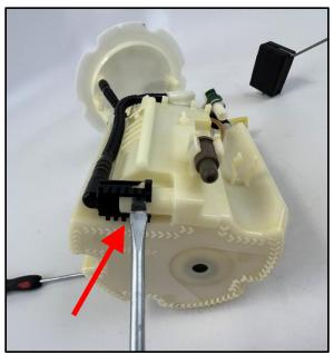
19. Release the (3) tabs securing the pump assembly housing to the lower basket (1 tab shown below). Then lift up to remove the pump assembly from the basket.
