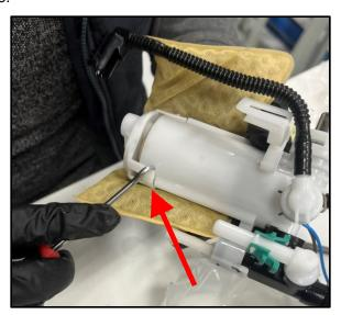
21. Remove the OE fuel pump from the pump assembly housing. Once removed disconnect the electrical connector at the top of the OE fuel pump.
