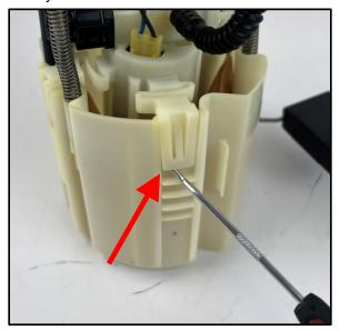
20. Release the (3) locking tabs securing the fuel pump strainer to the bottom of the fuel pump and then remove the strainer and set aside.
