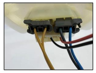
17. Release the tab and then lift up on the fuel level sending unit to remove it from the basket.
