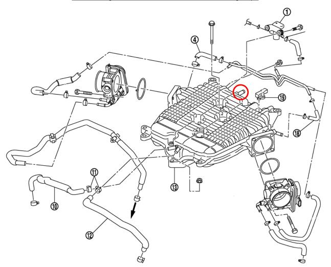
13. Loosen hose clamps (1) and remove OEM PCV Breather hoses (10) & (12) at the front of the intake plenum.
