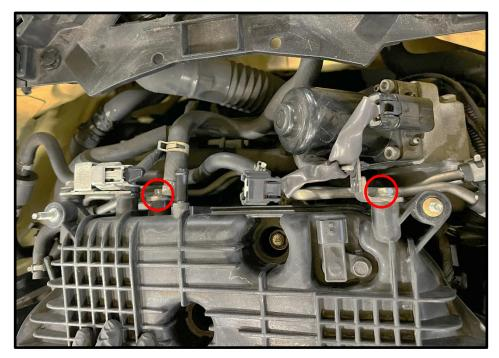
20. Remove (8) nuts and bolts securing intake plenum to engine in reverse order as shown in figure below.
