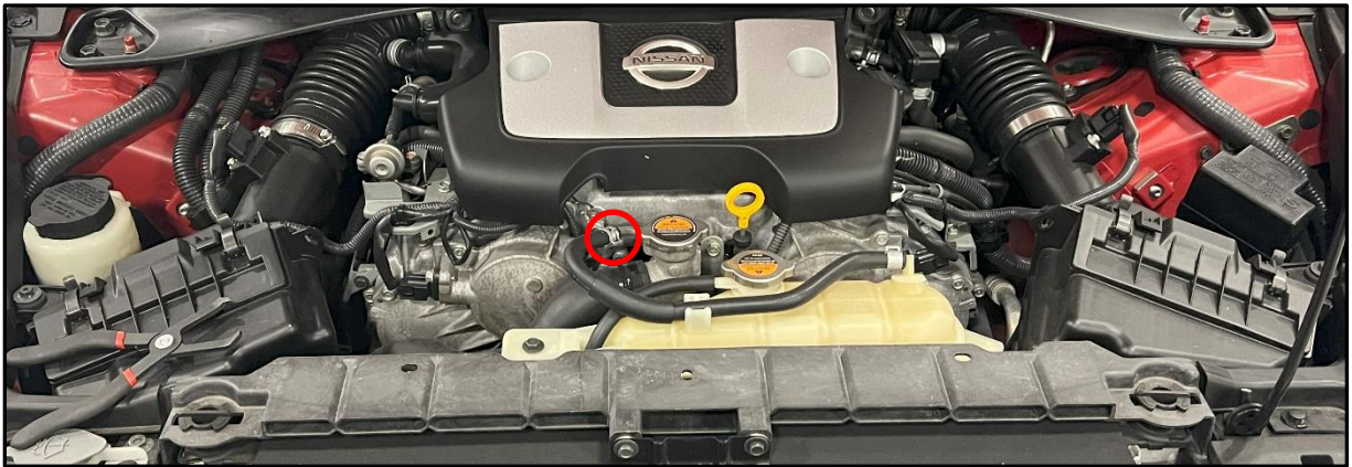
(late style is car is shown above, but coolant neck location is the same)
