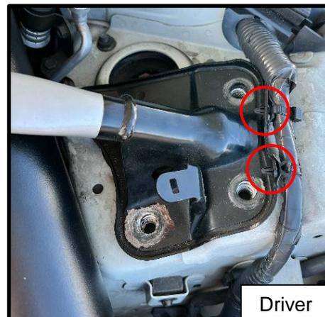
5. Remove the strut tower brace and set aside.
