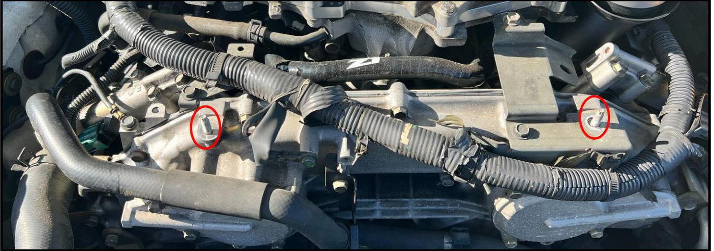
Note: The picture above shows the mounting holes with the factory studs installed.
