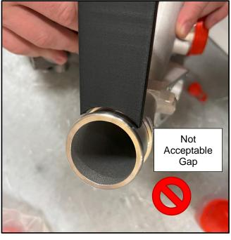
5. If you notice a considerable gap or that the "nub" doesn't sit flush in the coolant feed port with the (2) holes lined up on the exhaust inlet flange, you need to slightly clock the turbine housing.
