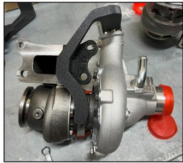
3. With the (2) bolt holes on the exhaust inlet flange lined up, hold the fixture and exhaust inlet flange together and check the nub to make sure it is sitting nicely in the coolant feed port.
