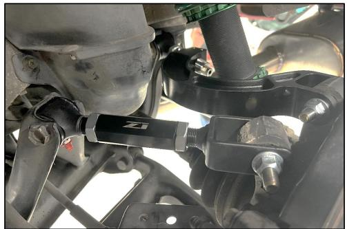
Note: If equipped with street version bushings, assure serviceable grease fittings face downwards.
