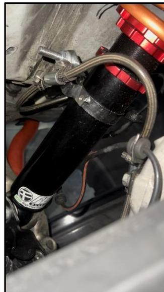
23. Final tightening of components going through rubber bushings should be completed when the vehicle is on the ground. Torque specs can be found below, under the instructions for the rear.
