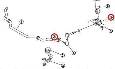
9. Remove the (3) bolts securing the brackets to the backside of the lower control arms (circled below). Remove brackets and set aside.
