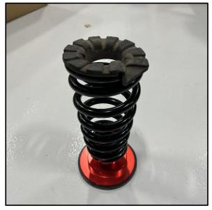
35. Starting on one side of the vehicle, position the spring and spring collar assembly into the toe arm spring bucket so that it sits flush on the bottom of the arm. The step in the spring and lower rubber seat will match up with a step in the toe arm spring bucket.
