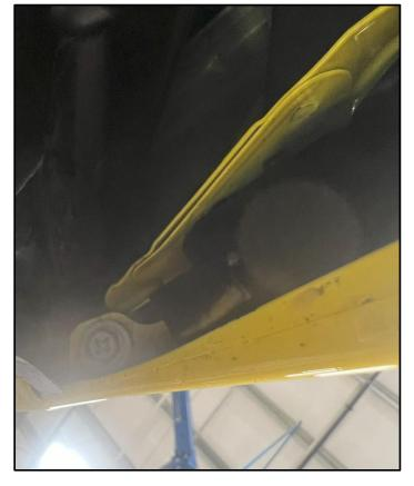
11. There are (2) electrical connectors on a bracket in the passenger side of the bumper (shown below). Disconnect both of them. The image below is shown with the bumper already removed.
