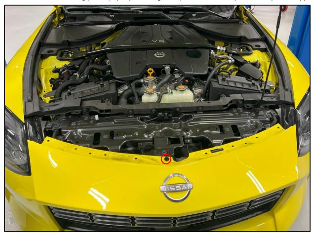
10. Remove the screw on each corner of the bumper securing it to the front of the fenders.
