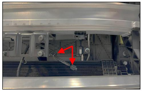
17. Remove the (2) bolts and (2) nuts securing the crash beam to the vehicle.
